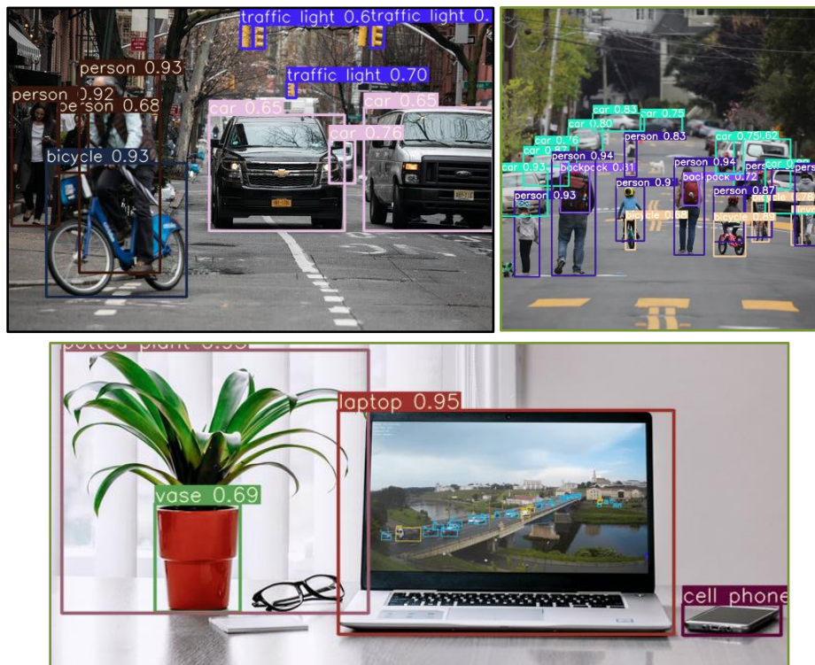
Figure 6. YOLOv7 results on the COCO test set calculated using saiwa object detection online interface. Bounding boxes are shown in color in addition to categories, and confidences.
