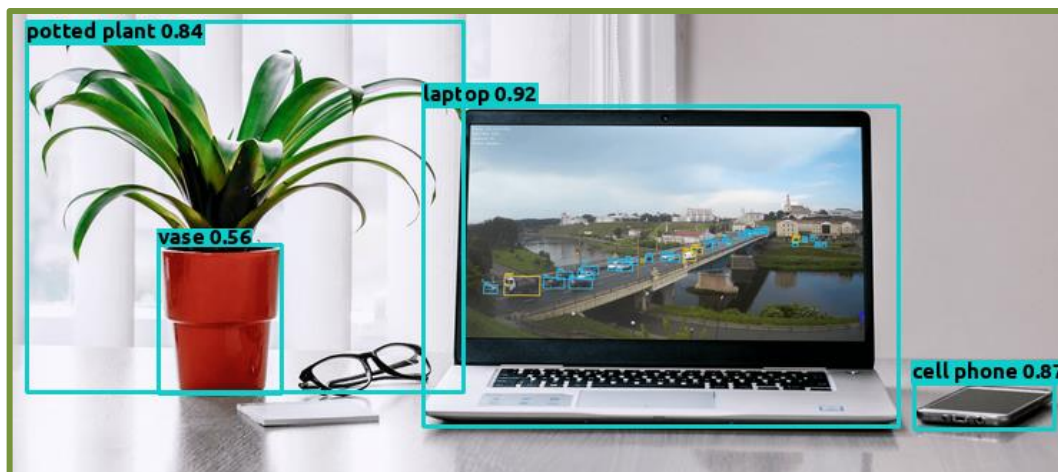
Figure 3. YOLOv5 results on the COCO test set calculated using saiwa object detection online interface. Bounding boxes are shown in color in addition to categories, and confidences.
