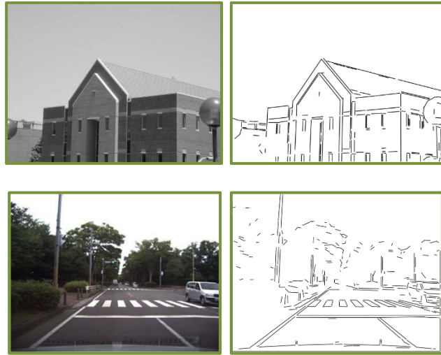
Figure 1. LSD results on natural images using saiwa Line Segment Detection service interface.
